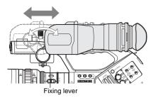
Tighten the fixing lever after the adjustments.
